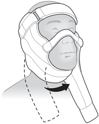
Figure 8.4.c. Adjust Right Inner Chin Flap Under Chin
